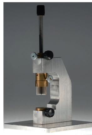
Figure 2. Study-specific cutting device with orthogonally mounted surgical blades and engaging carrier allowing standardized cutting of replicas.
